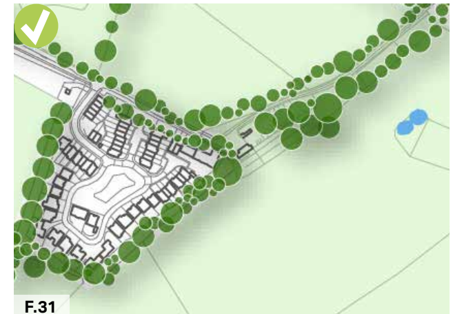
Figure 31: Diagram of a positive treatment of the edges in a development surrounded by a green buffer that offers a smoother transition into the open fields
